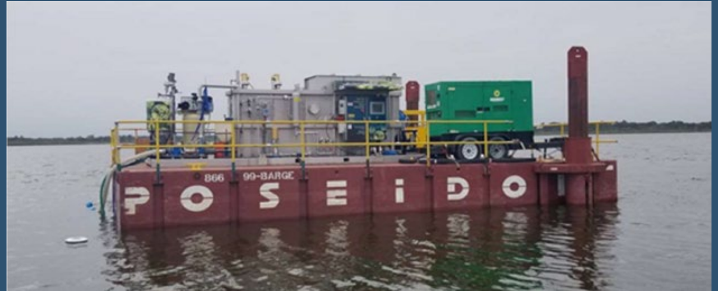
Algae harvester with Hydronucleation Flotation Technology AECOM Technical Services Inc.
